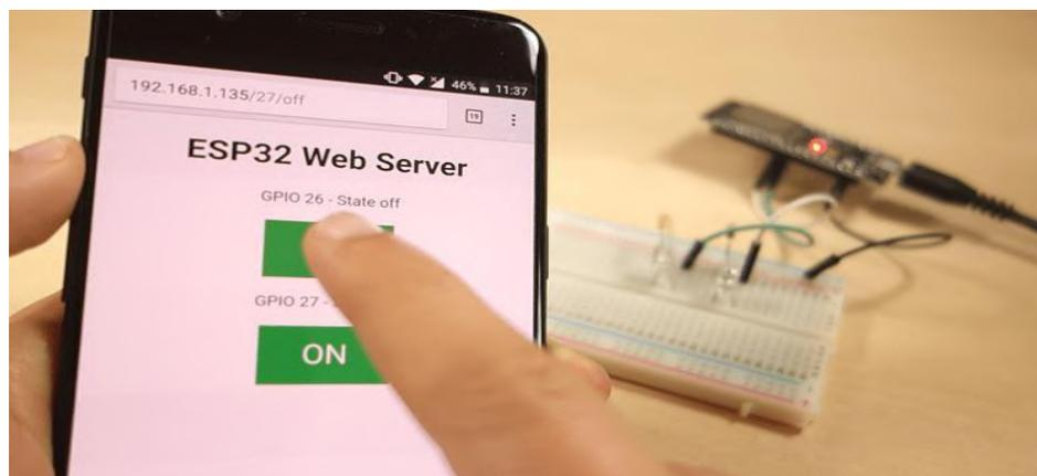
At the same time, you can take a look at the Serial Monitor to see what's going on in the background. For example, when you click the button to turn GPIO 26 ON, ESP32 receives a request on the `/26/on` URL.
