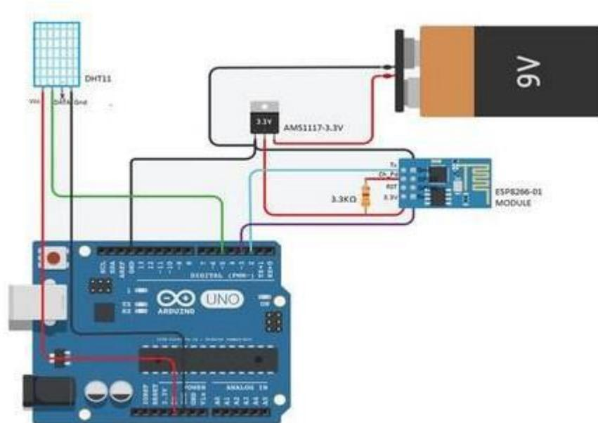
Fig 1.1: Circuit diagram for monitoring Humidity and Temperature in IOT cloud
