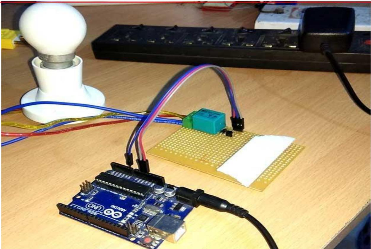
**Working** is simple, we need to **make the RELAY Pin (PIN A0) high to make the Relay module ON and make the RELAY pin low to turn off the Relay Module.** The AC light will also turn on and off according to Relay.
