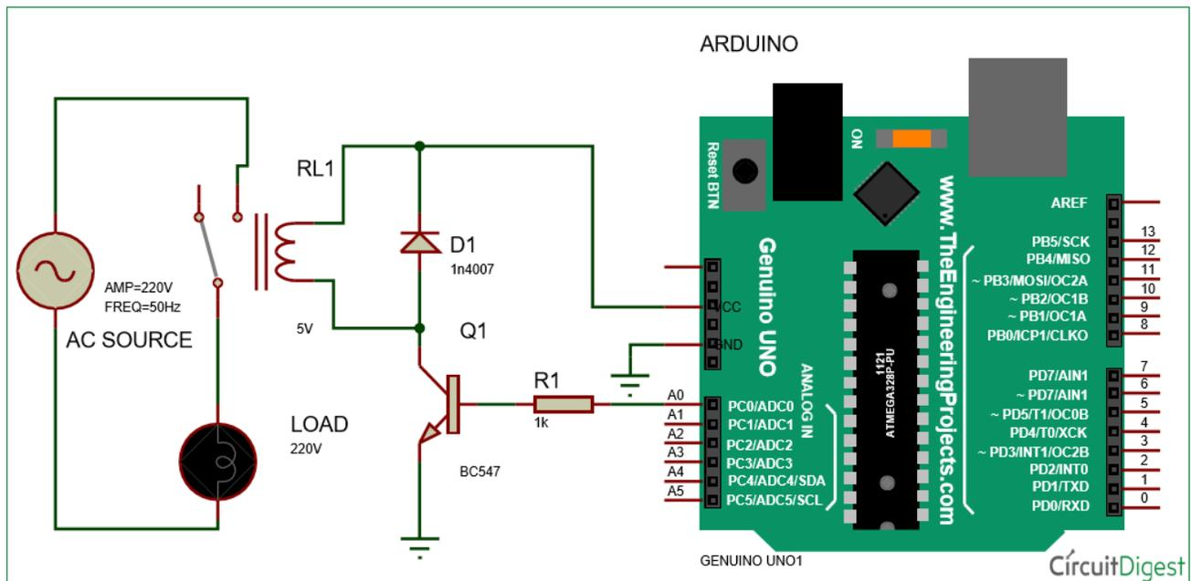
In this **Arduino Relay Control Circuit** we have used Arduino to control the relay via a BC547 transistor. We have connected transistor base to Arduino pin A0 through a 1k resistor. An AC bulb is used for demonstration. The 12v adaptor is used for powering the circuit.
