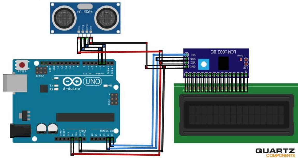
Trig and Echo pins of the ultrasonic sensor are connected to digital pin 3 & 2 of Arduino.  $V_{CC}$  pin of the ultrasonic sensor is connected to the 5v pin of Arduino while the GND pin is connected to the GND of Arduino. SDA & SCL pin of the I2C module is connected to the A4 & A5 pin of Arduino while  $V_{CC}$  and GND pins are connected to the 5V & GND pin of Arduino.
