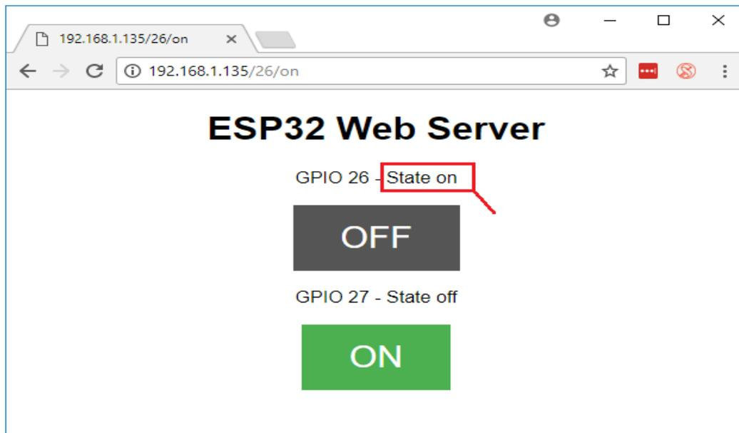
The button for GPIO 27 works in a similar way. Test that it is working properly.
