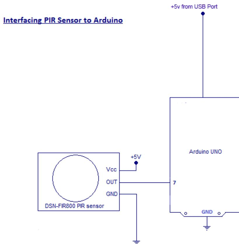
**PIR Sensor** – is the heart of this simple burglar alarm circuit using arduino. A PIR sensor – is basically a motion sensor or a motion detector which identifies any object
