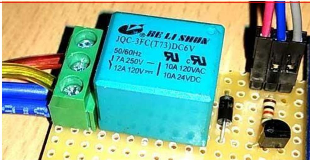
Here to **turn on the Relay with Arduino** we just need to make that Arduino Pin High (A0 in our case) where Relay module is connected.
