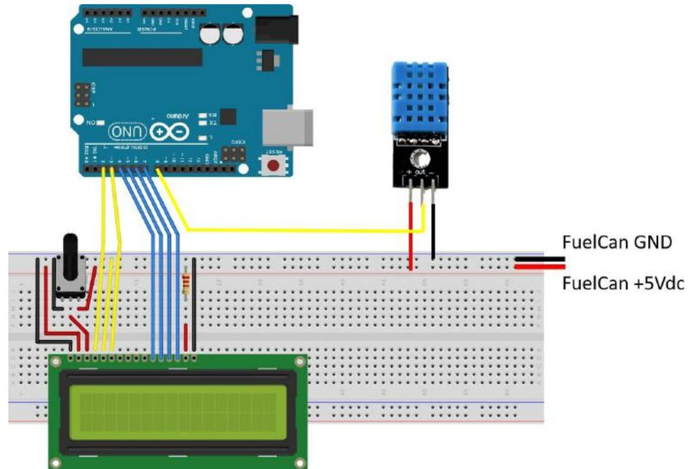
Interface 16x2 LCD to Arduino by connecting pins 4,6, and 11-14 of the LCD connected to Uno pins 2,3, and 4-7, respectively. Connect the LCD using a solderless breadboard.
