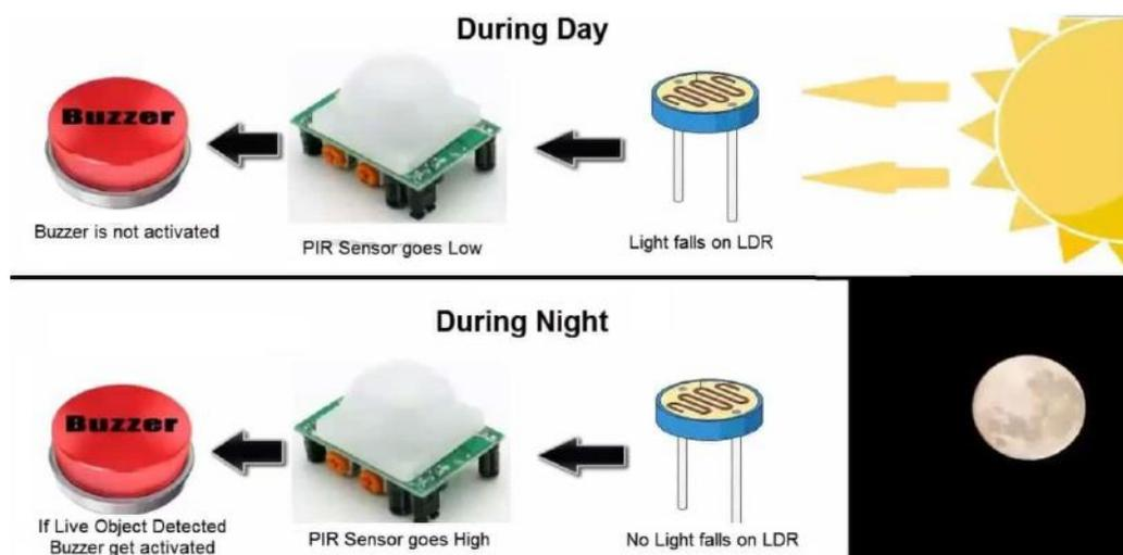
The best sensor you can use to detect an intrusion is the Passive Infrared (PIR) Sensor. The PIR Sensor detects the motion of a human body by the change in surrounding ambient temperature when a human body passes across, and effectively controls the switching when it detects a moving target.
