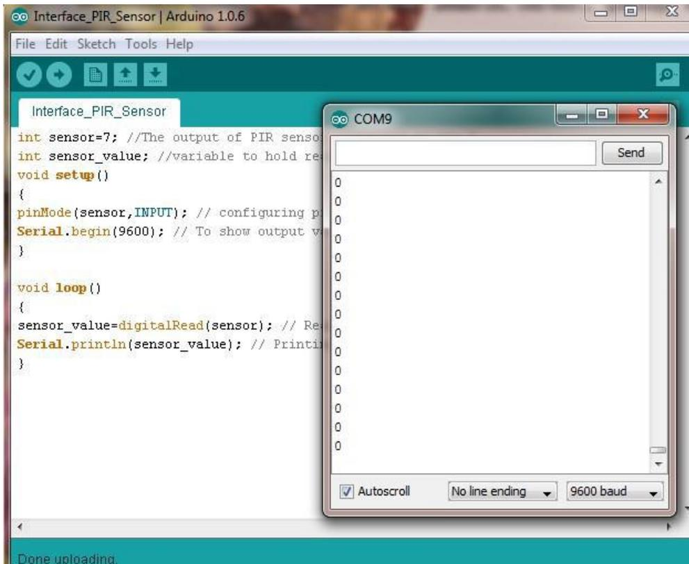
Output of PIR Sensor in Arduino Serial Monitor – when there is motion detected in range
