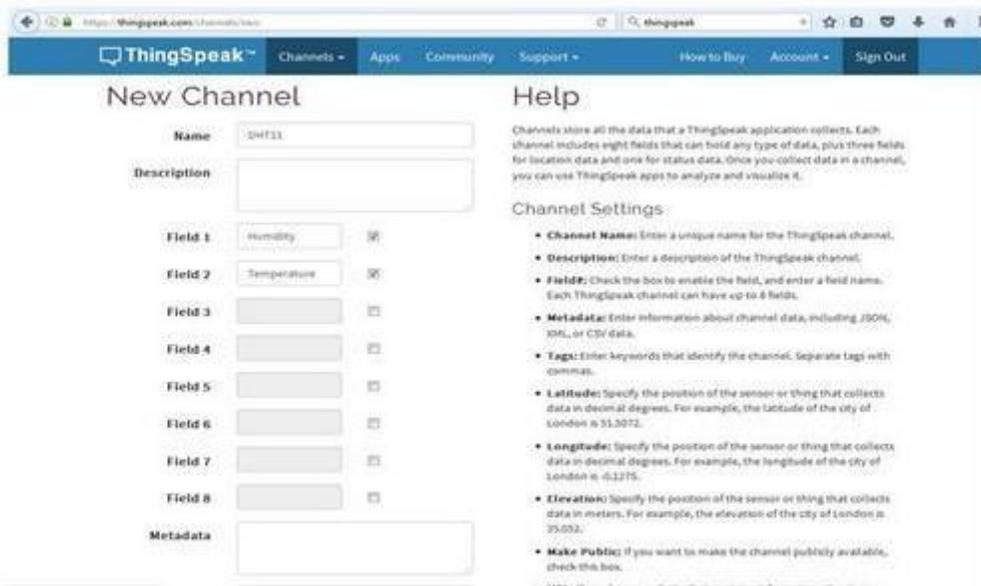
Fig. 1.2: Creating new channel on ThingSpeak cloud
